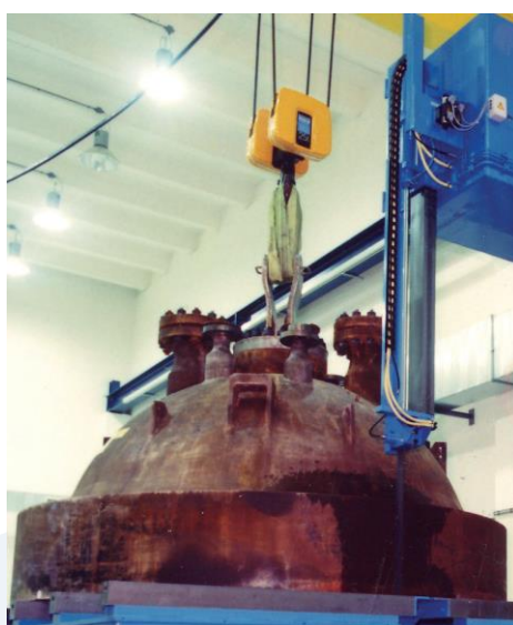
Figure 10 : Band saw with a dual-column guide
