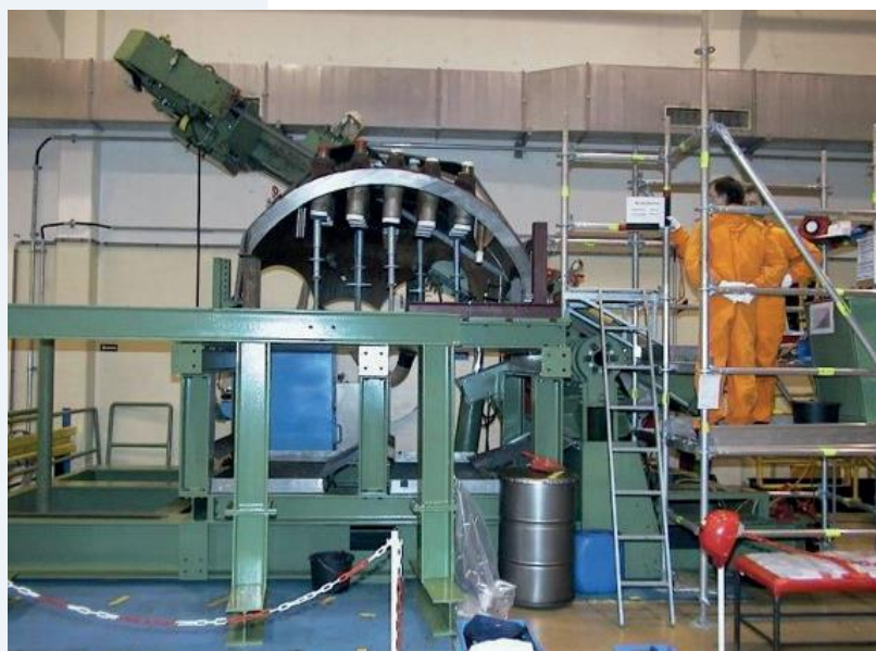
Figure 9 : Band saw with swing frame
