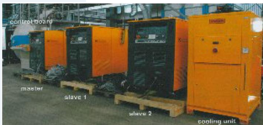
Figure 5 : Plasma power sources with control board cooling unit and supply lines
