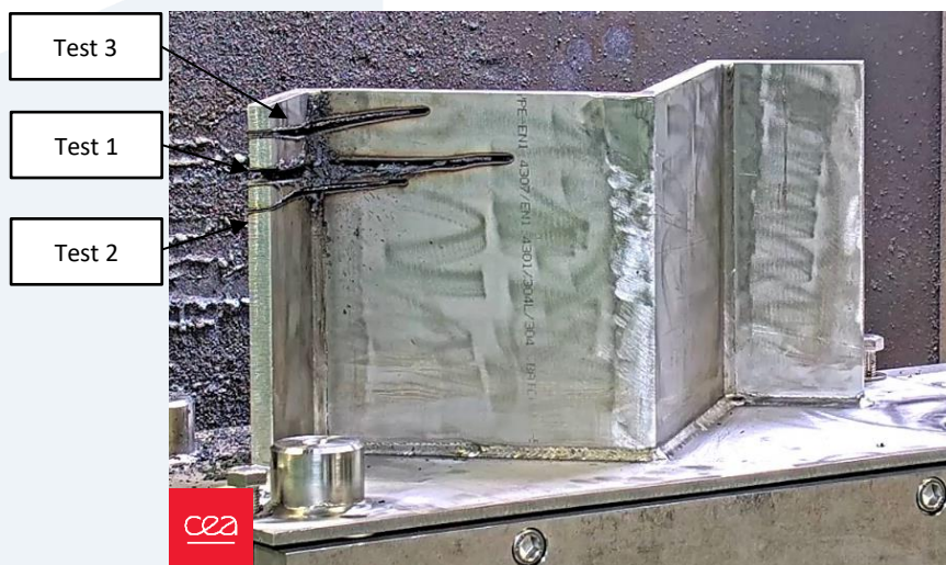
Figure 49: Result core shroud tests (concave part with collection device)
