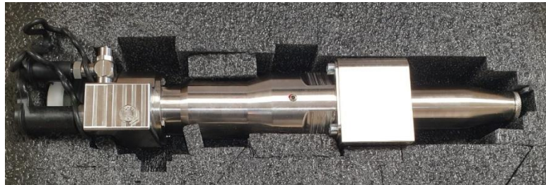
Figure 5: In-air laser cutting head
