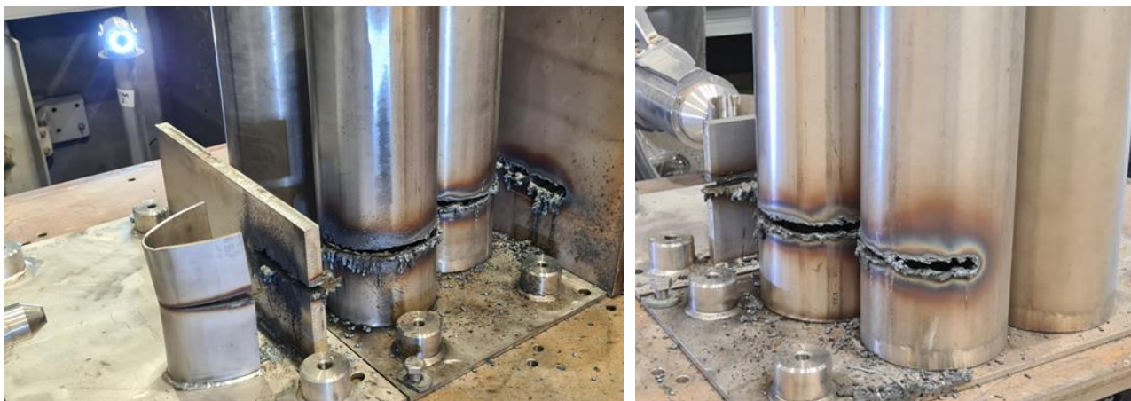
Figure 98: Result two steam dryers tests with internals, support ring and core cover (Front view and rear view)
