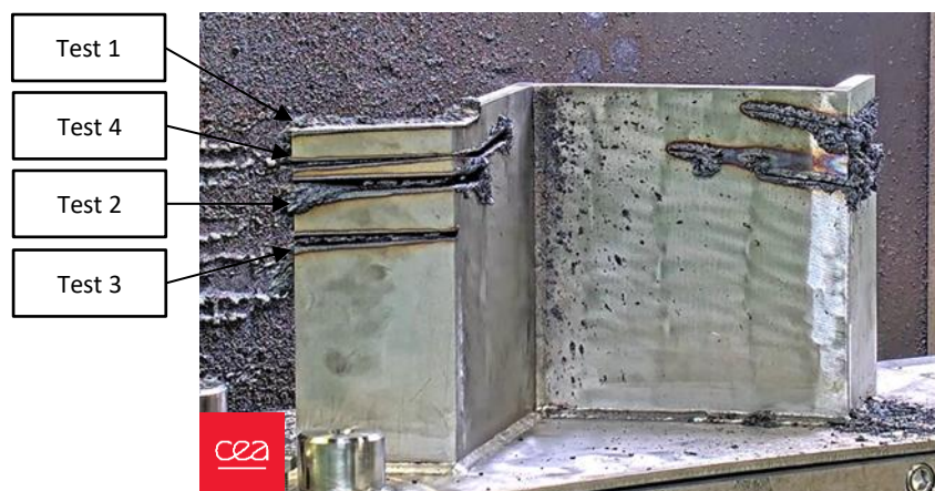
Figure 44: Result core shroud tests (convex part with collection device)
