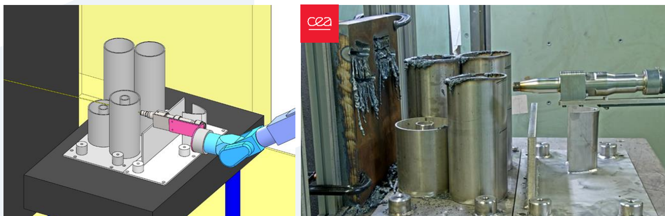
Figure 57: Steam dryer configuration before testing
