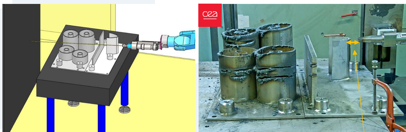
Figure 66: Steam dryers with internal, support ring and core cover configuration before testing
