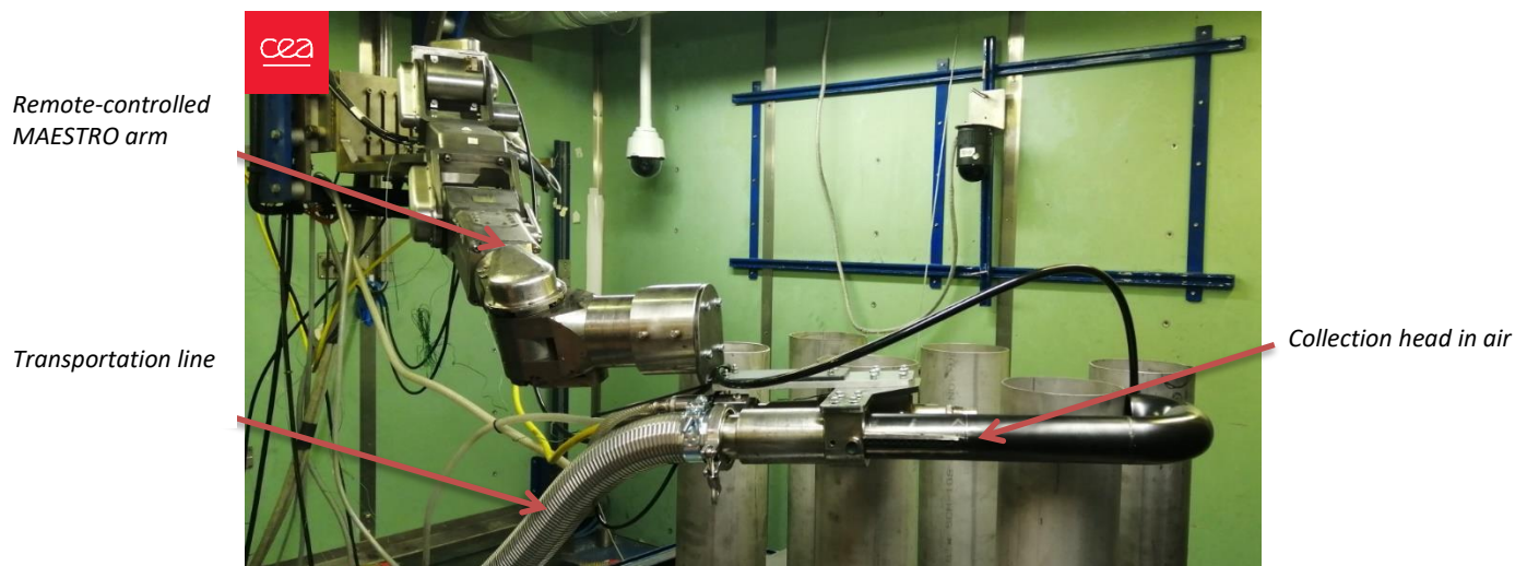
Figure 6: In-air laser head on MAESTRO arm (HERA Facility)
