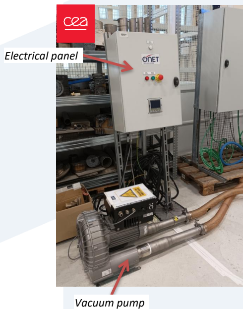
Figure 8: Collection device in control area
