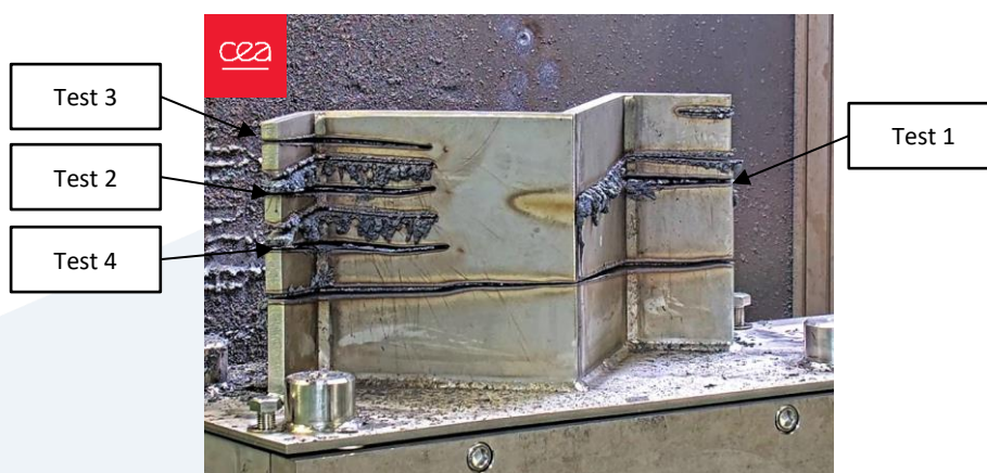
Figure 47: Result core shroud tests (concave part)
