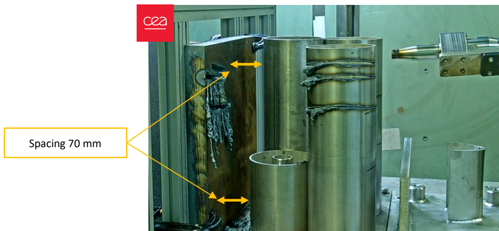
Figure 81: Martyr plate test configuration
