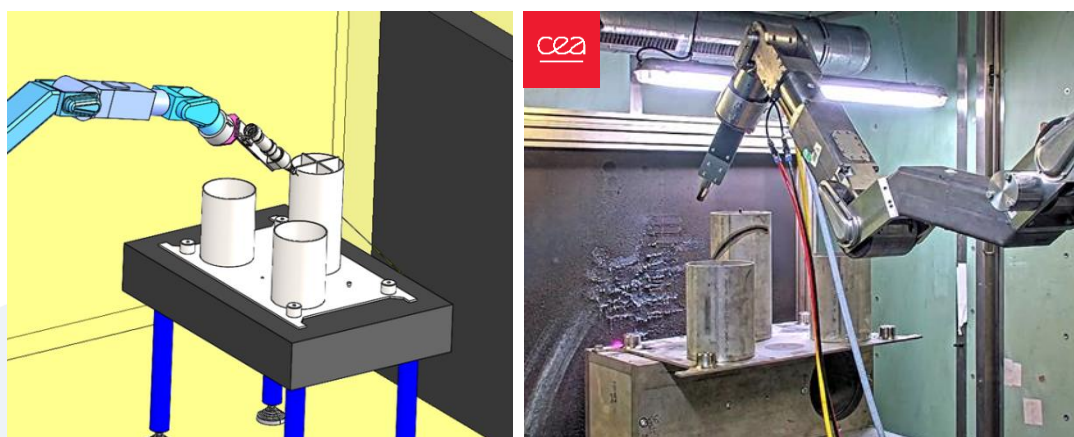
Figure 74: Control rod with poisoning plate configuration before testing (45° angle)
