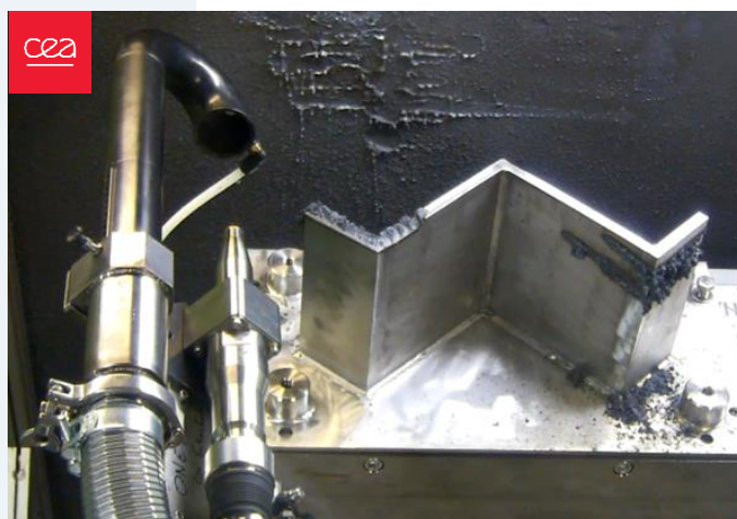
Figure 43: Core shroud configuration before testing with collection device
