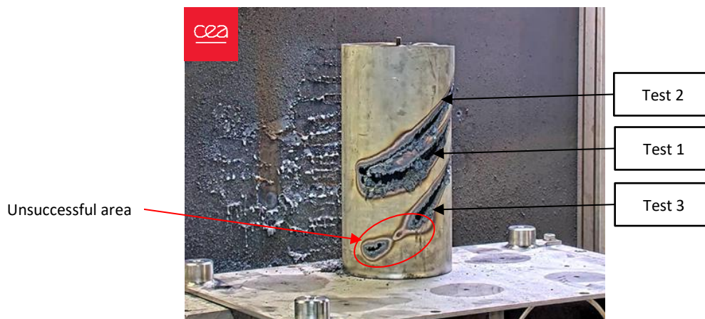
Figure 75: Result control rod with poisoning plate 45° angle tests (Front and rear view)
