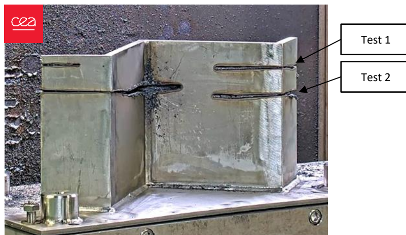
Figure 42: Result core shroud tests (convex part)
