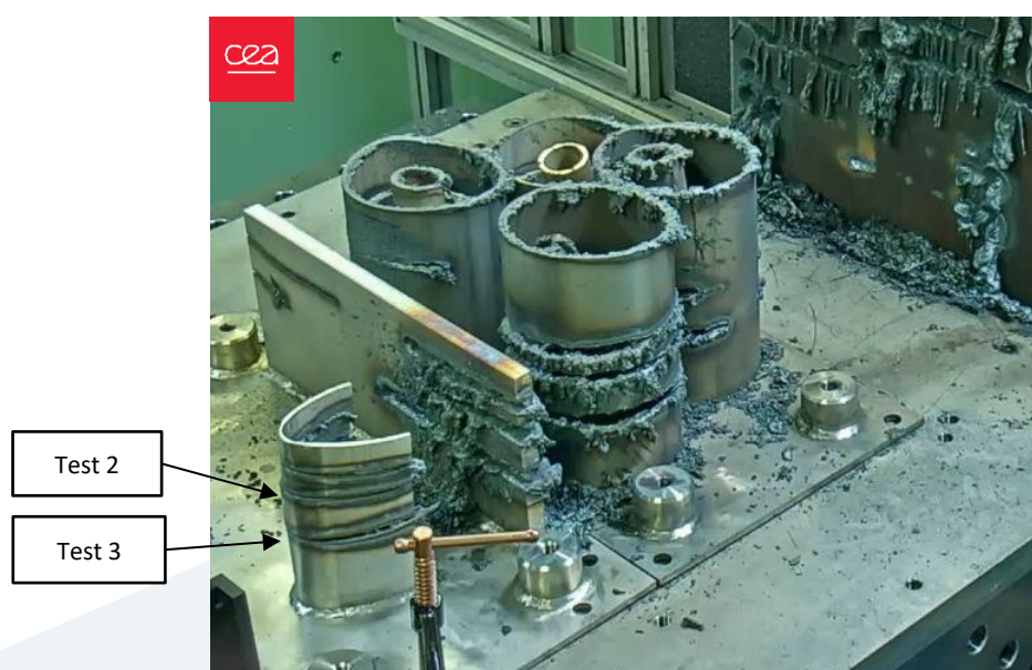
Figure 67: Result two steam dryers tests with internals, support ring and core cover (Front view)
