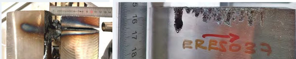
Figure 5. Example of cutting on 304L stainless steel with sample in background (left) and cross-section of the sample in the background showing blind kerf (right)
