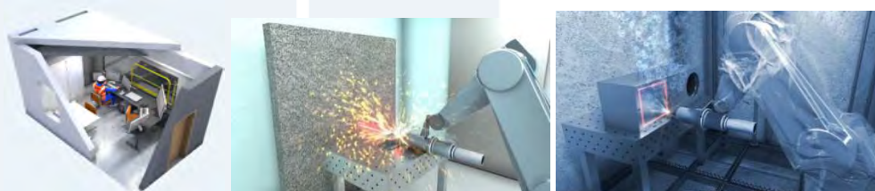
Figure 16. Illustration of in-air and underwater cutting operation during demonstrators
