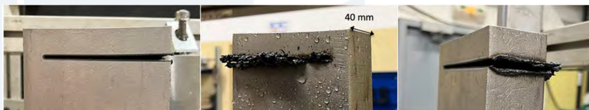
Figure 10. Laser underwater cut performed on a 40 mm stainless steel 304L at 8kW
