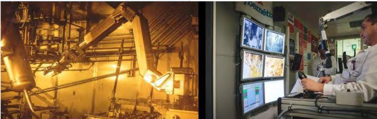
Control room operator (right) controlling the Maestro robot arm in a Marcoule pilot unit (APM) cell (left).
