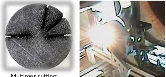
Multipass cutting: 60 mm thick graphite @ 8kW
