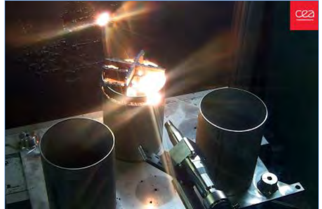
In-air laser cutting of mock-up (BWR Steam Dryer and Core Cover) at HERA Facility (CEA Marcoule). Source: CEA.
